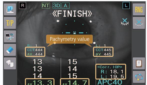
The pachymetry data can be used to display a corrected IOP value.
