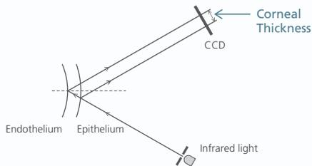
The principle of specular reflection for pachymetry allows a more compact design of TONOREF™ III.
